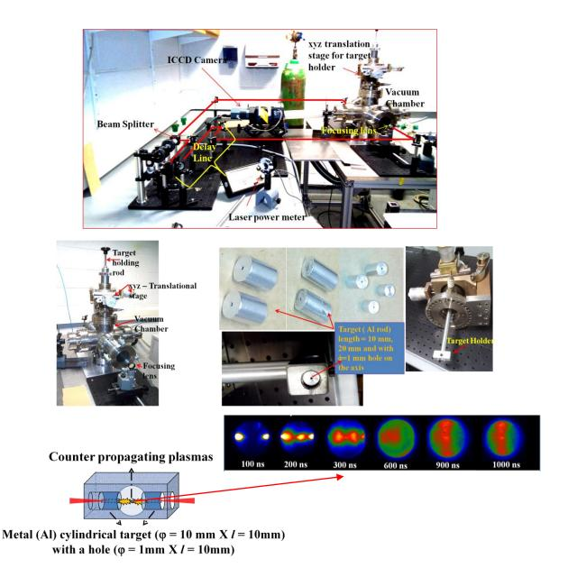
Fig. 1 Schematic diagram of the experimental setup and target design and schematic diagram of the focusing of a laser beam into the target hole and collision of horizontally opposed plasmas and formed stagnation layer.
