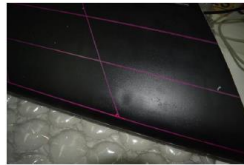
Figure 20. Visible damage due to impact with the 50mm hailstone.
