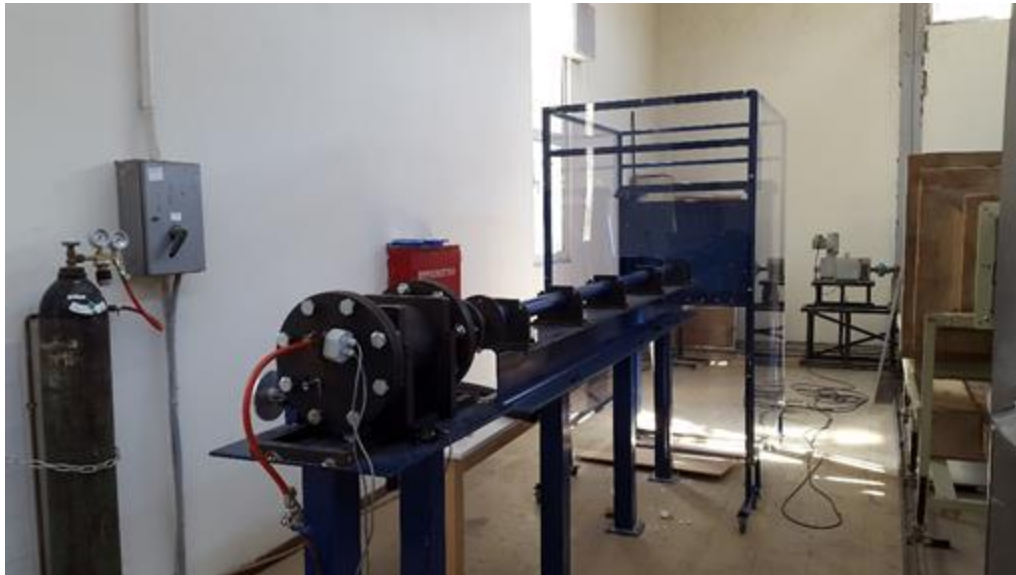
Figure 4. The fully assembled impact gun including the safety precautions
