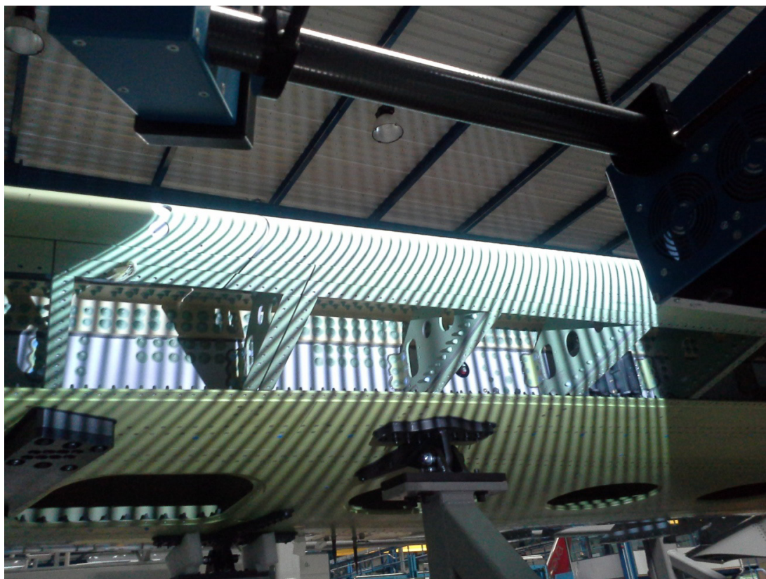
Figure 2: Fringe-projection measuring procedure applied to the BLADE GKN wing (front nose section & lower cover)
