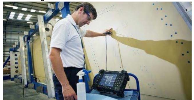
Figure 5: Manual NDT Inspection
