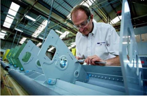
Figure 11: Inspection of GKN Machined LE Assembly
