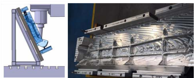
Figure 10: LE Section Machining Jig (Left) and LE Section Roughing Out (right)
