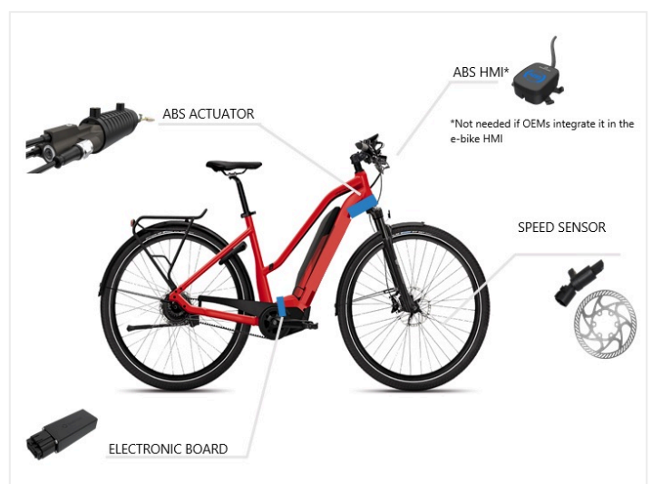
BluBrake components and their positioning on the bike
