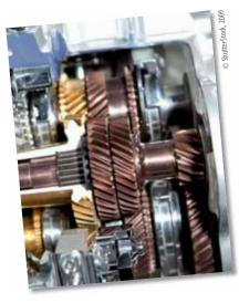
Coated components are very frequently used in tribological systems, in which surfaces of two parts are in moving contact with one another — as is the case in the automotive industry. Coatings allow for wear reduction and at times, lighter materials provide technical solutions for conforming to emerging emission laws.
