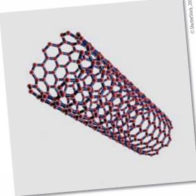
Carbon nanotubes are ultra-thin fibres of carbon and a nanotechnologist's dream. They are made from thin sheets of carbon only one atom thick, known as grapheme, rolled into a tube only a few nanometres across. Even the thickest is more than a thousand times thinner than a human hair.
